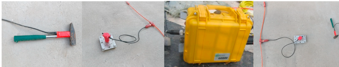
(a) Hammer (b) Receiver (c) Seismograph (d) Monitoring line
